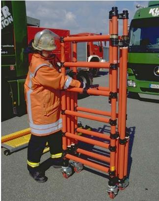
1. Unlock the brakes of the swivel castors
