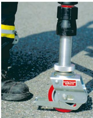
7. Block the swivel castor or check the base plate for secure stand
