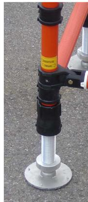
8. Adjust the rescue platform by height adjustment with quick lock, check the lock again
